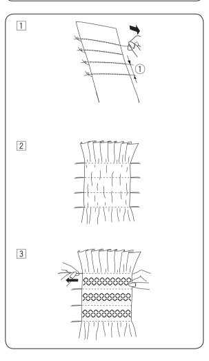
1 Choose a soft and lightweight fabric such as batiste, gingham or challis. Cut the fabric three times wider than the project width. Increase the stitch length to "4" and loosen thread tension to "1". Sew rows of straight stitches 3/8" (1 cm) apart across the area to be smocked.
