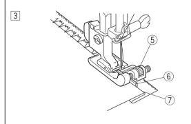
3 Turn the screw to align the guide on the foot with the folded edge so that the needle just pierces the fold.
