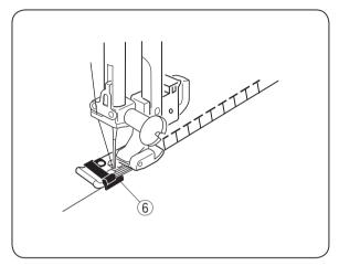
This stitch is ideal for finishing edges of stretch fabrics. It seams and finishes the fabric edges simultaneously.
