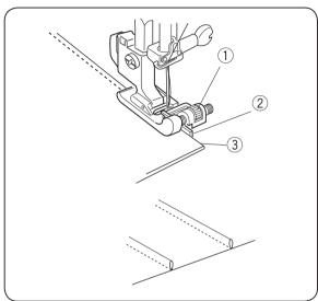
Fold a fabric wrong side together. Lower the needle into the fabric 0.1-0.2 cm inside the folded edge.
