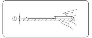
To check needle straightness, place the flat side of the needle onto something flat (a needle plate, glass etc.) The gap between the needle and the flat surface should be consistent.
