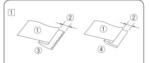
1 On heavy weight fabrics that ravel, the raw edge should be overcast first.
