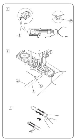
With the buttonhole foot raised, hook the filler cord on the spur at the back of the foot. Bring the ends toward you under the foot, clearing the front end. Hook the filler cord into the forks on the front
