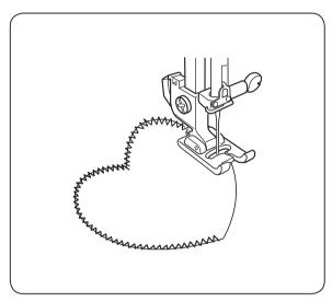
Baste appliqué pieces on the fabric, or fuse the appliqué pieces with an iron-on fabric joiner. Stitch around the appliqué, making sure the needle at the right swing falls along the outer edge of the appliqué.
