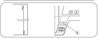
Use this stitch to secure the beginning and the end of a seam with backstitching.
