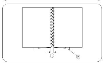
Use this stitch to join two pieces of fabric to create an open work appearance and add design interest. Fold under each fabric edge 5/8" (1.5 cm) and press. Pin the two edges to paper or tear backing 1/8" (0.3 ~ 0.4 cm) apart. Sew slowly, guiding the fabric so the needle catches the folded edge on each side. After finishing the sewing, take off the paper.
